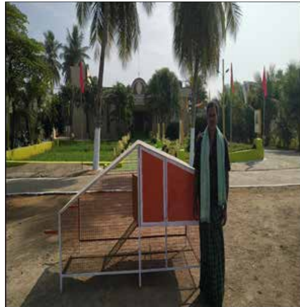
Duplex back yard poultry rearing unit for rearing securely 15-20 Poultry Birds
